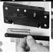
12. Attach the pair of steel VRS support brackets to the cast finger support brackets (with the horizontal surfaces inwards) using the four 10-24 button head screws and washers, but just finger tighten only.
