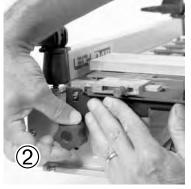
**9.** Loosen the support bracket knobs and while holding the board down flush on the finger assembly, raise one steel bracket until the "peak" ① on top of the VRS extrusion touches the underside of the board. Now tighten the knob at that end ②. Repeat at other end. Double check and readjust both ends as needed until the finger assembly is level with the VRS extrusion "peak" ①.
