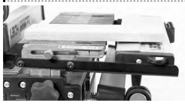
**13.** Mount the finger assembly and lower it onto its support board. Install the VRS onto the steel brackets and lay a flat board on the finger assembly, extending out over the top of the VRS extrusion.
