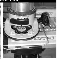
**16.** Install the two router follower rails by placing the wire ends into the selected holes as far as possible; then using thumb and index finger, squeeze and "snap" the arm down into the end of the slot. Position the wire brackets to allow routing of the work piece outer edges. Efficient waste collection does not require centering the router bit in the collector.
