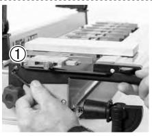
**10.** Now firmly tighten the two button head screws ①. The hex key stows in the right hand end of the VRS ②. After installation, when raising and lowering the combined
