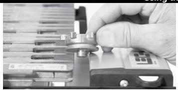
**17.** Adjust the VRS forward position to allow a gap between the extrusion and tips of the jig guide fingers (or template) that is greater than the guide bushing diameter used.
