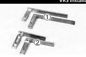
**5.** D4R Pro, D4R, D4 and 24" D3, D1258R & D1258 Owners: With the exception of the D4R Pro, first, remove the long support brackets ① from your jig (or short brackets from your D1258/R, not shown). Then, install the "new" short brackets ② included with the VRSD24. D4R Pro Jig Owners: The new brackets are identical to those supplied with your jig. Keep as spares.
